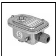
TYPE 09: Prefixes WP/WS: IP67, EM/WSEM: II 2 G/D, IP67, EEx em II, WPDU/WSDU: II 3 D, IP67, T85°C to 200°C, WPZN/WSZN: II 3 G/D, IP67, EEx nA II, WPIS: II 2 G/D EEx ia IIC Low power Steel, epoxy coated (EM, WP, WPDU, WPZN, WPIS) AISI 316 SS (WS, WSDU, WSEM, and WSZN) IEC 335 / EN 50019, EN 50028 and 50281-1-1
