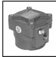
TYPE 08: Prefixes NF/NL/WSNF: II 2 G/D, IP67, EEx d IIC Low power Aluminium, epoxy coated (NF) Cast iron, epoxy coated (NL) AISI 316 SS (WSNF) EN 50018 and EN 50281-1-1
